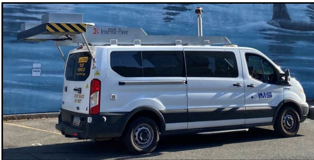
Figure 1 - IMS Integrated Road Information System platform (IRISPro Pave)
