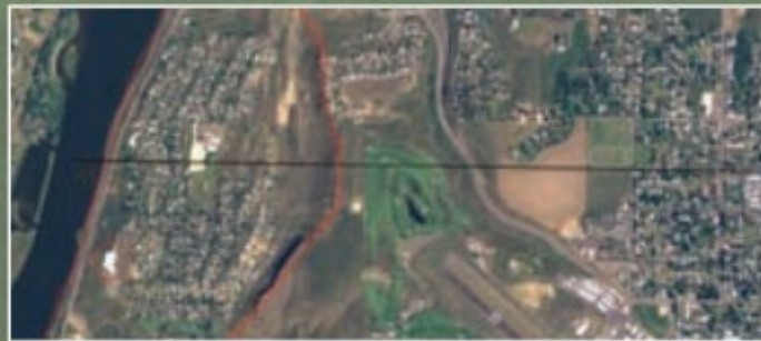
Air photo of landslide complex along the Snake River near Lewiston. The landslide is outlined in red. Location of the geologic cross-section is shown by black line. The white building in lower left is the Elks Lodge, site of a smaller landslide.
