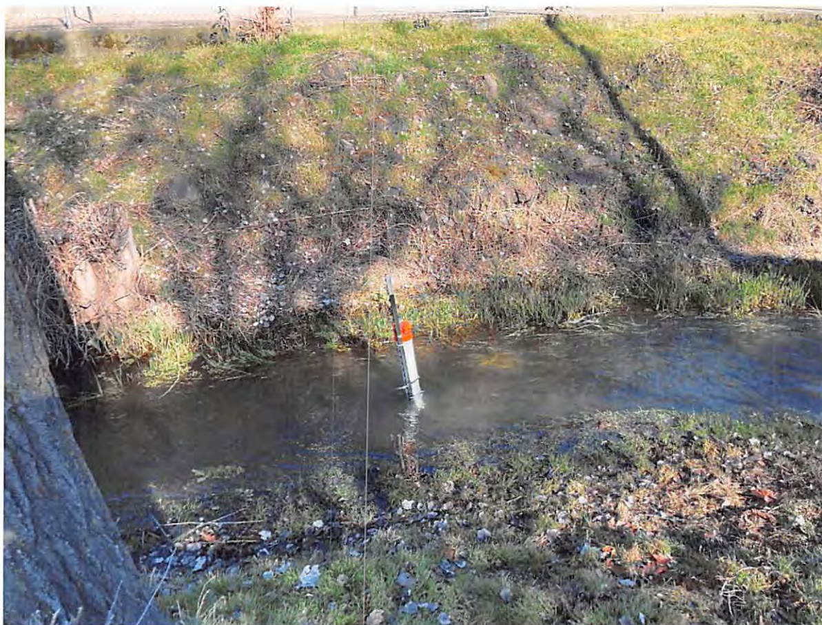
Figure D-3. EXO2 casing deployed in Lindsay Creek.
