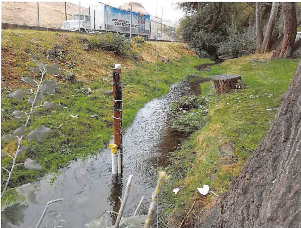
Figure 2. Lindsay Creek in-stream monitoring station, equipped with data logging pressure transducer.
