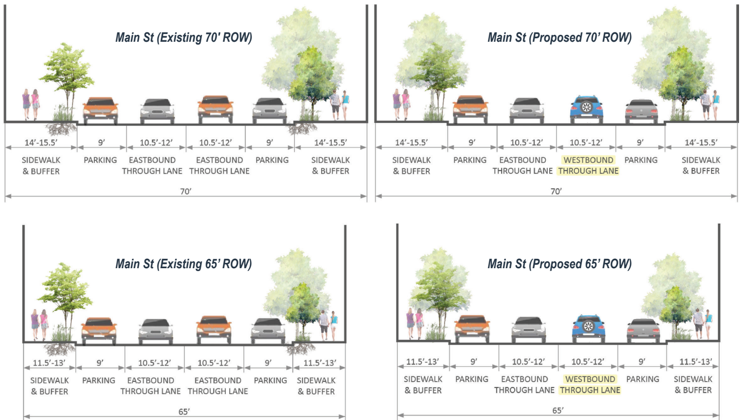
Figure 3. Existing Main Street and Proposed Two-Way Main Street Cross Sections
